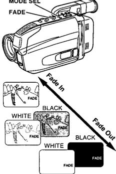
If FADE is accidentally pressed, press again so that "FADE" disappears in the EVF.
