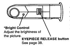
\*Note: These controls have been set at the factory. It is not necessary to adjust these controls under normal circumstances. But, should it become necessary, be careful to make the adjustment with a small, slender screwdriver so as not to damage the miniature control.
