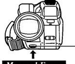
For Auto Focus mode, it may be necessary to **press MANUAL FOCUS**, so that "MF" does not appear in the EVF.
