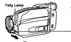
Set the POWER switch to CAMERA. Built-In Lens Cover opens.
