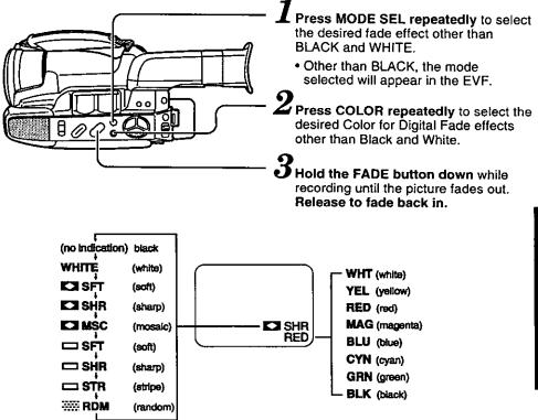
■ To create even more special effects, (other than BLACK, WHITE, and RANDOM modes), you may also partially fade the picture, and by pressing the MODE SEL button, freeze the fade function. Press FADE again to resume, or press MODE SEL to cancel.
