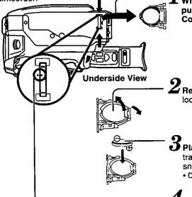
While pinching the stopper tabs, pull the tray out of the Battery Compartment.
